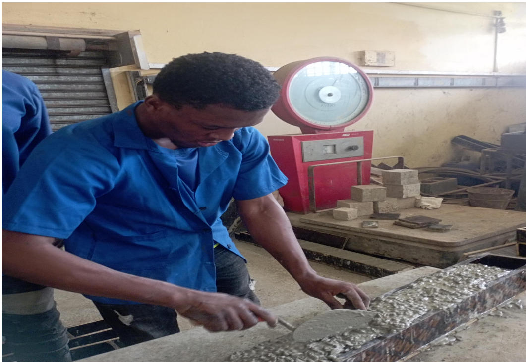
Figure A2: Moulding of concrete cubes
