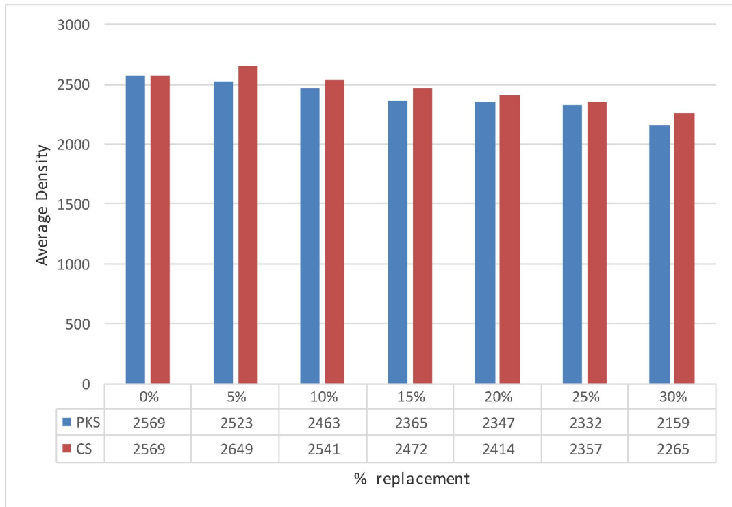
Figure 4.4a Comparison on Average Density of concrete made with Palm Kernel shell and Coconut shell.
