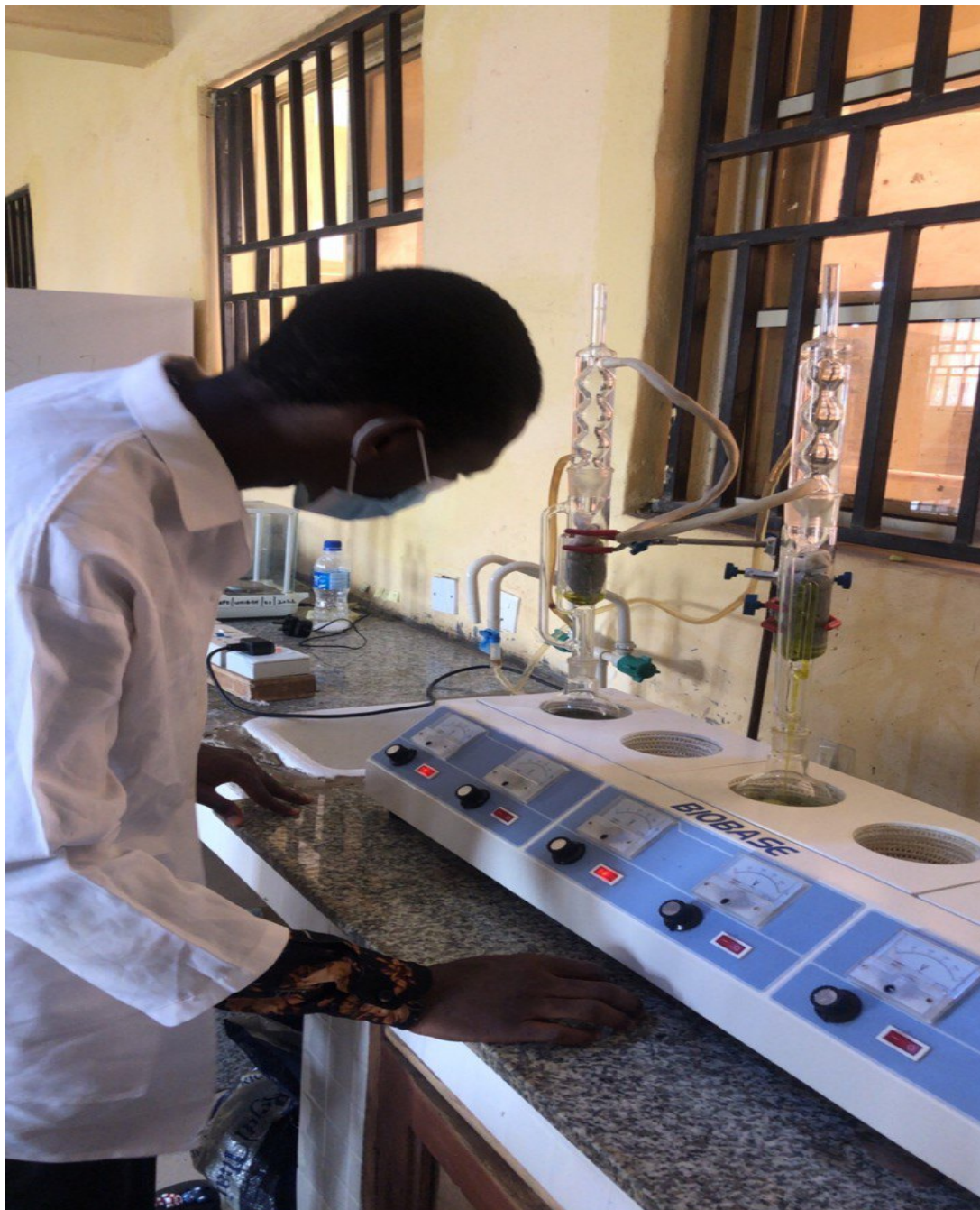
Plate 2: Soxhlet Extraction Setup
