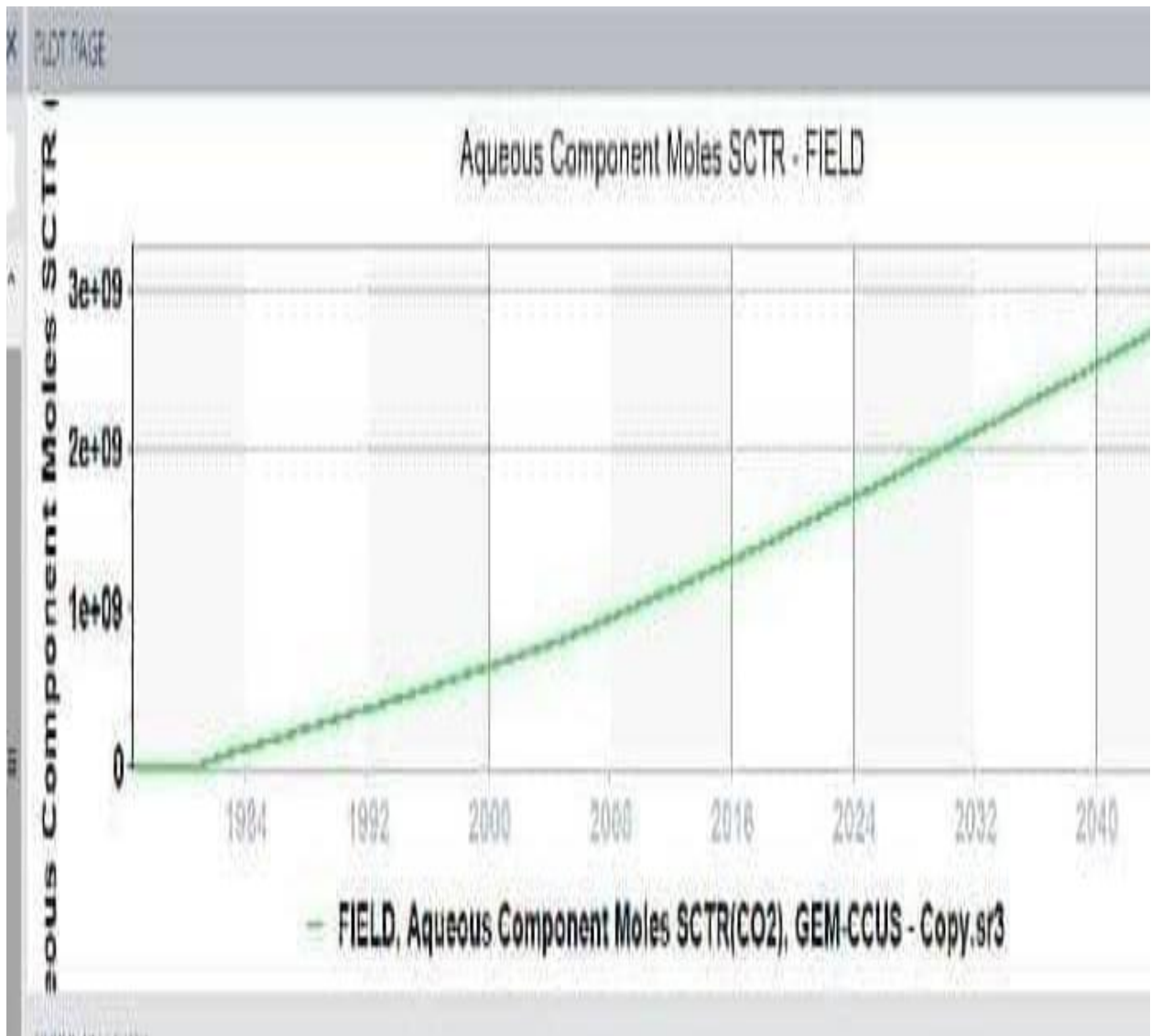
Figure 4.1: Variation of Aqueous CO 2 Moles in the Reservoir from 1976 to 2045
