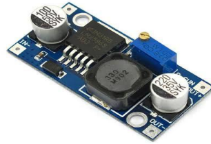
Figure 3.9 - LM2596 Buck Converter DC-DC Step Down Power Module
