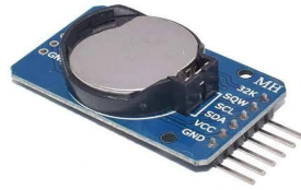
Figure 3.6 - A DS3231 Real Time Clock (RTC) Module
