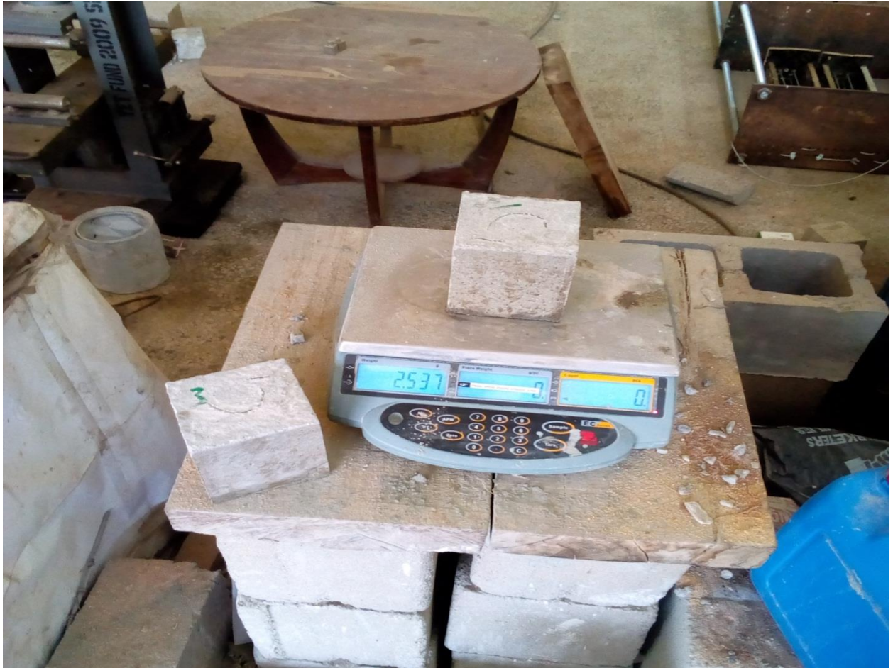
Weighing the mass of concrete
