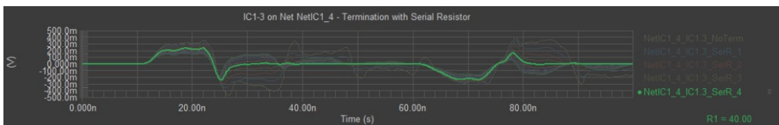
Figure 4.9: Simulated crosstalk for differential microstrip without termination
