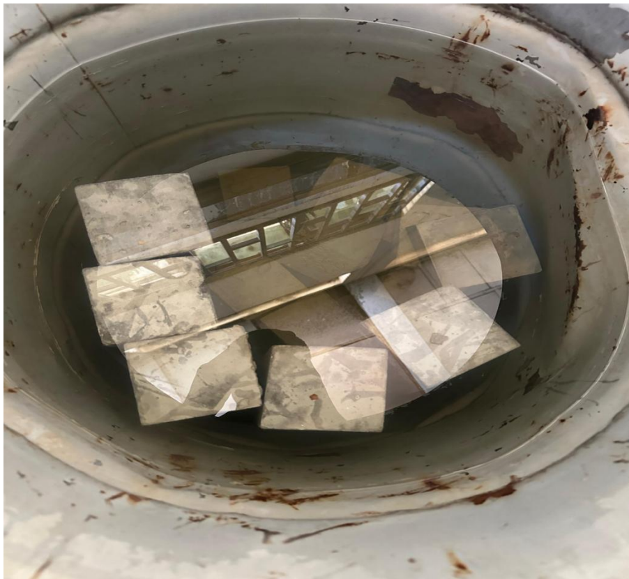
Plate A-5 curing of Cubes
