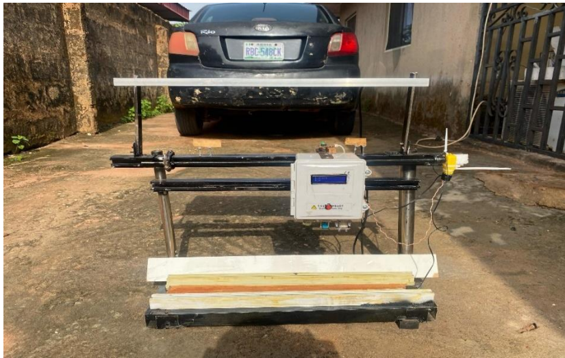
Figure 3.14 Field deployable wireless sensor network
