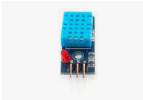
Figure 3.6 Humidity sensor module
