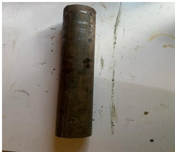
Figure 3.16 The corrosion free low Carbon Steel Pipe
