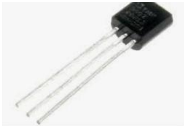
Figure 3.5 The lm 35 Temperature sensor
