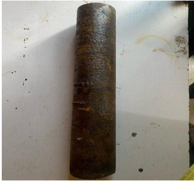
Figure 3.17 The corroded low carbon steel pipe
