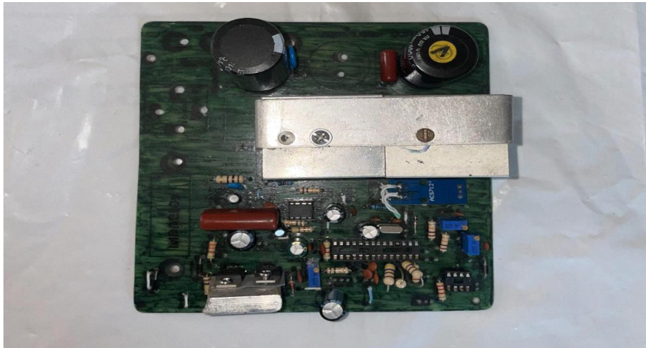
Figure 4.7: CHARGE CONTROLLER BOARD (MPPT)
