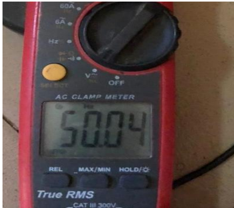
Figure 4.15: FREQUENCY OF OUTPUT VOLTAGE FOR LOCAL INVERTER
