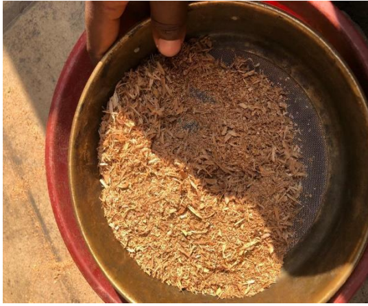
Plate 3. 2: Sample of sawdust been sieved
