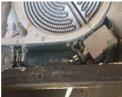
Figure 26 Heat Resistant Conductor for Internal Wiring
