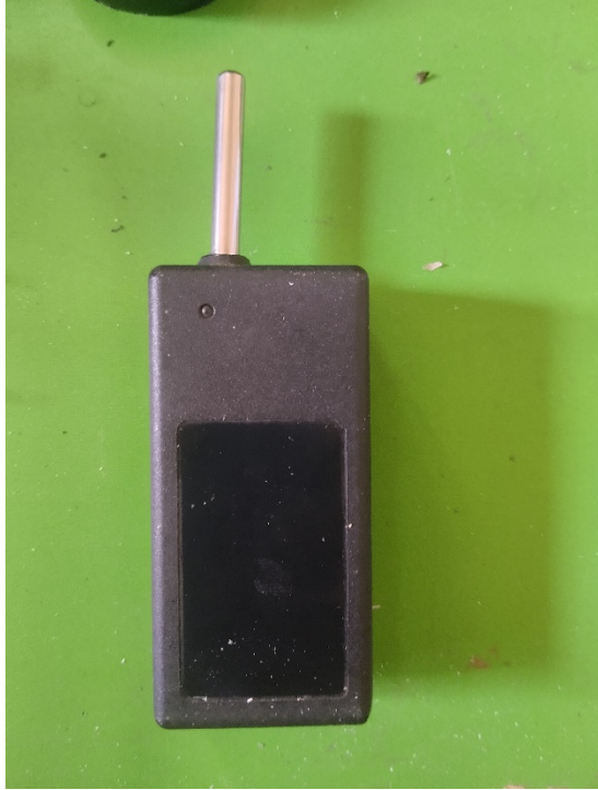
FIGURE 4,1 THE PIGGING DEVICE WHICH CONTAINS THE MICONTRROLLER(ESP 8266) AND THE SENSOR.
