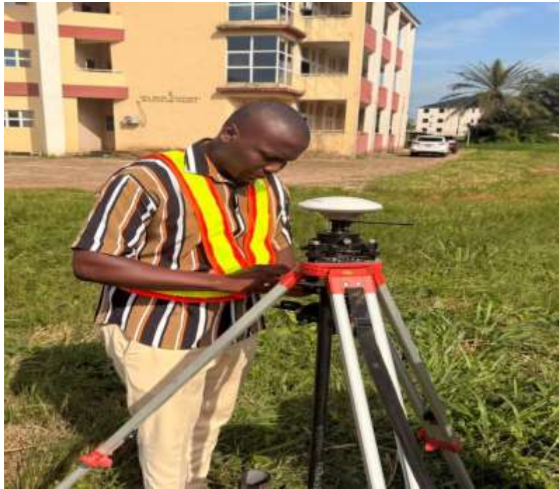
Fig. 3.8: GNSS Static Data Collection
