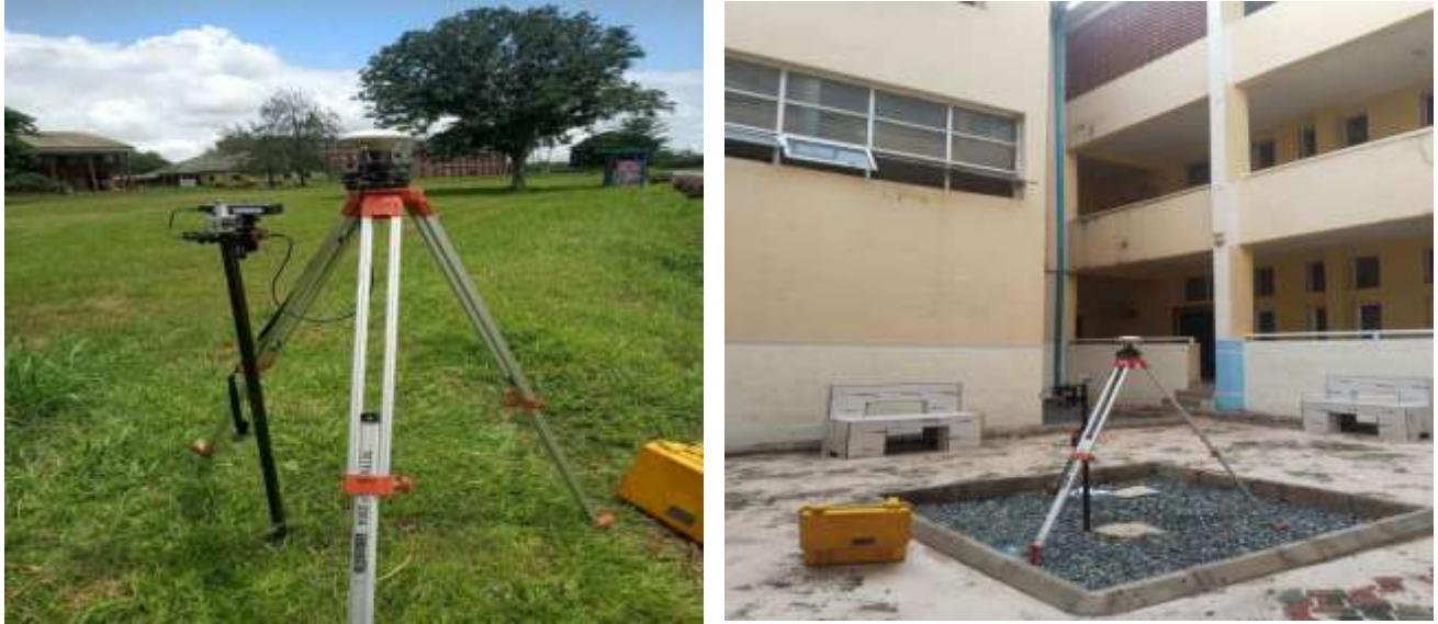
Fig. 3.7: Tersus David30 GNSS Equipment Setup at open-sky and multipath environment
