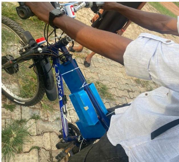
Figure 3.10: Testing of the Electric Bicycle after modifications are completed.
