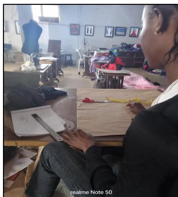
Pattern drafting and cutting of the Jacket Agbada garment
