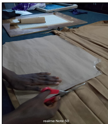
Pattern drafting and cutting of the Jacket Agbada garment
