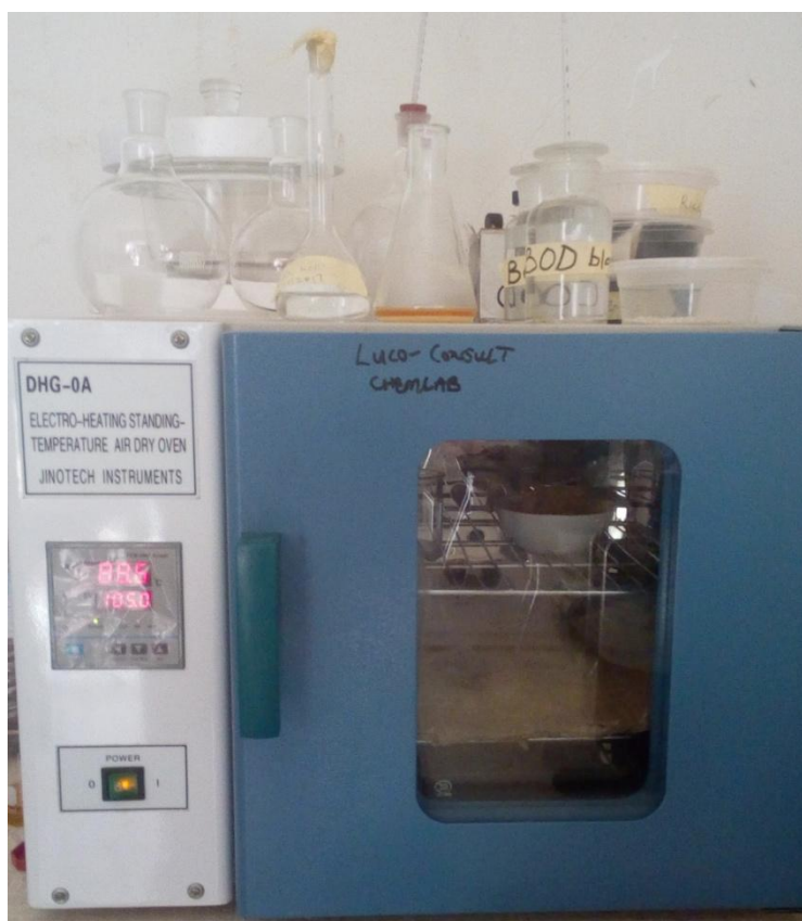
Figure 3.5 Drying of spent grain with an air drying oven
