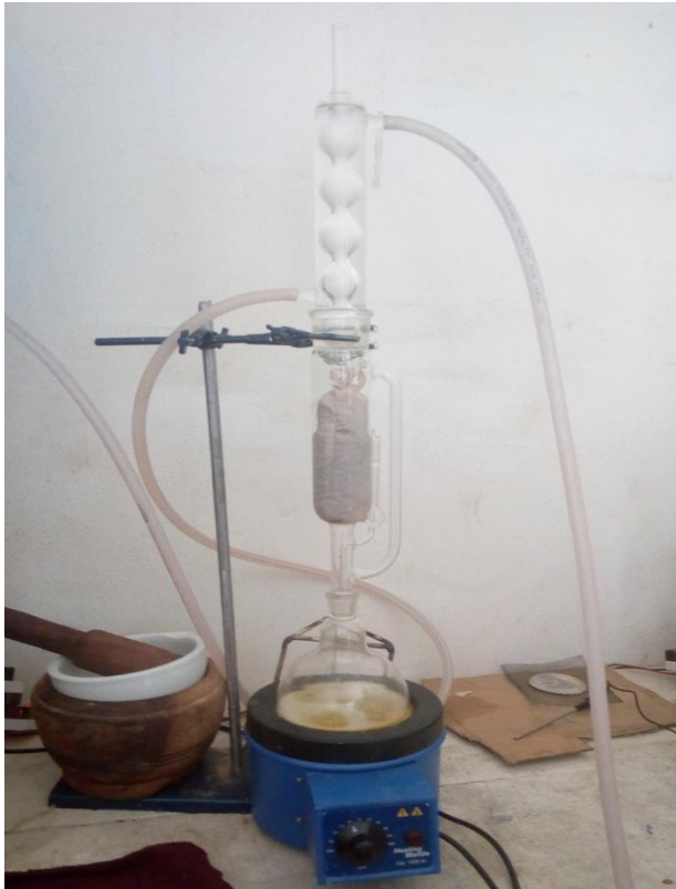
Figure 3.2 dewaxing of spent grain
