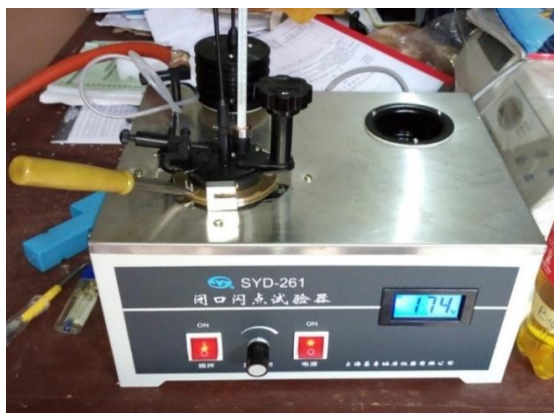
Figure 3.2: SYD-261 Pensky Martens Closed Cup Flash Point Tester
