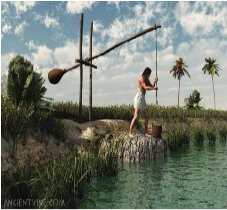
FIGURE 2.1 SHADUF USED FOR IRRIGATION IN EGYPT
