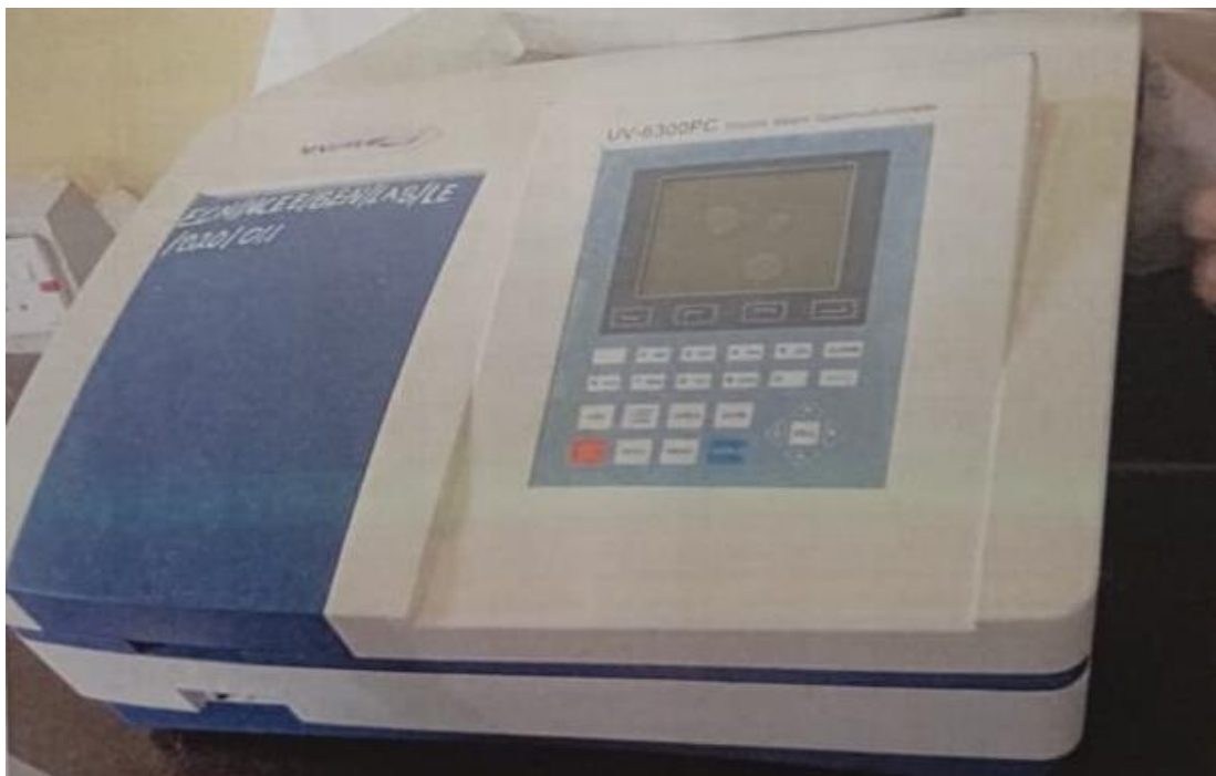
Fig3.3: T80+UV/VIS Double Beam Spectrophotometer
