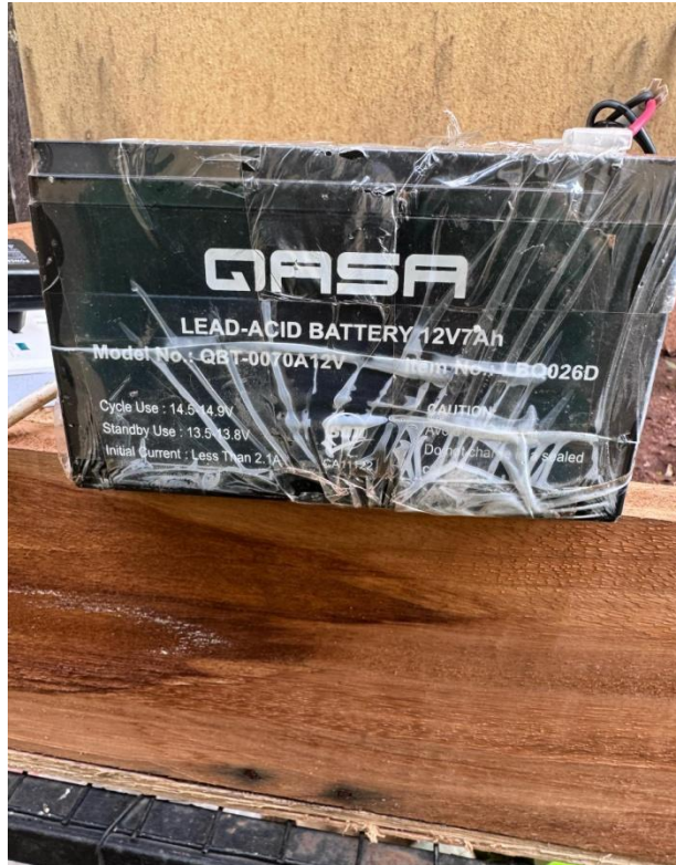
Figure 3.5: Battery to power the system
