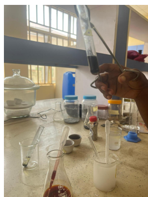
Fig 2.9: Iodine test for starch
