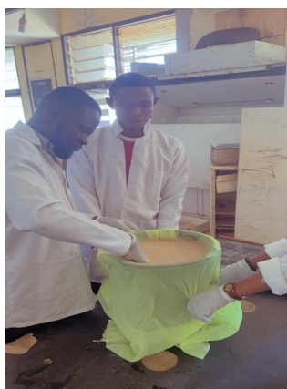
Fig 2.5: Filtration to collect starch
