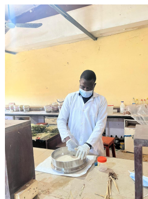
Fig 2.7: Sieving the dried starch with 125micrometer mesh
