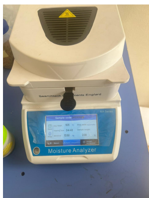
Fig 2.8: Moisture content determination for starch
