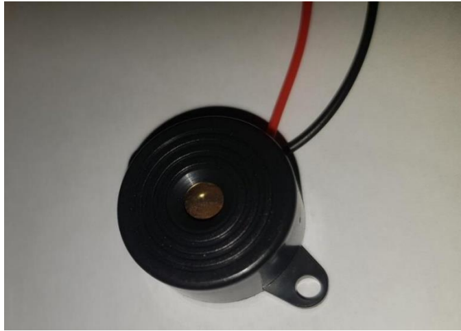
fig. 3.4 highdecibel3-24vdc active buzzer
