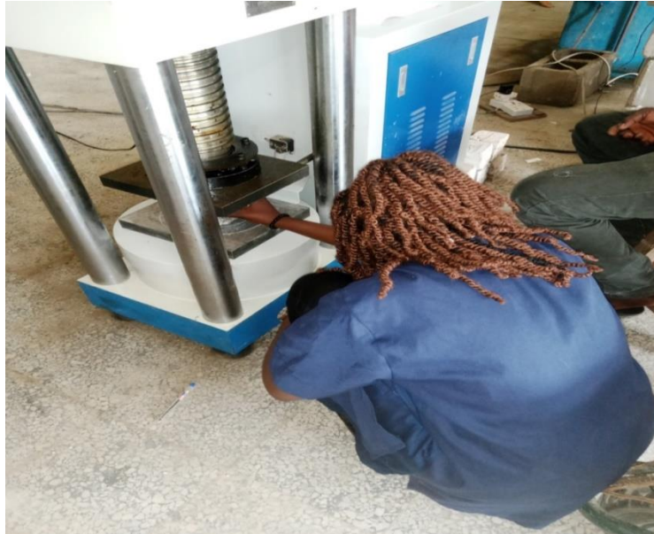
Figure 3.9a: Testing the compressive strength of the concrete cubes
