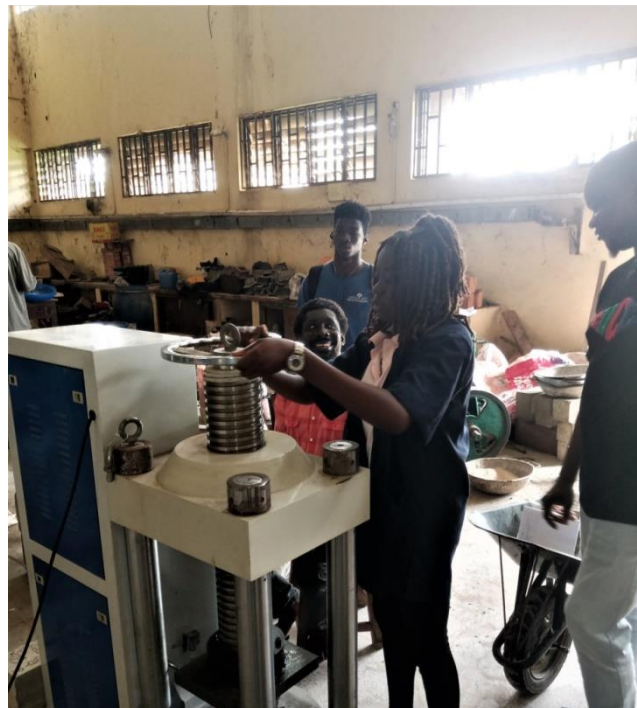
Figure 3.9b: Testing the compressive strengths of the concrete cubes
