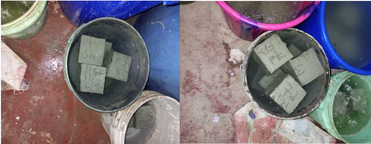
Figure 3.8: Curing of Concrete cubes in Bucket using potable water.
