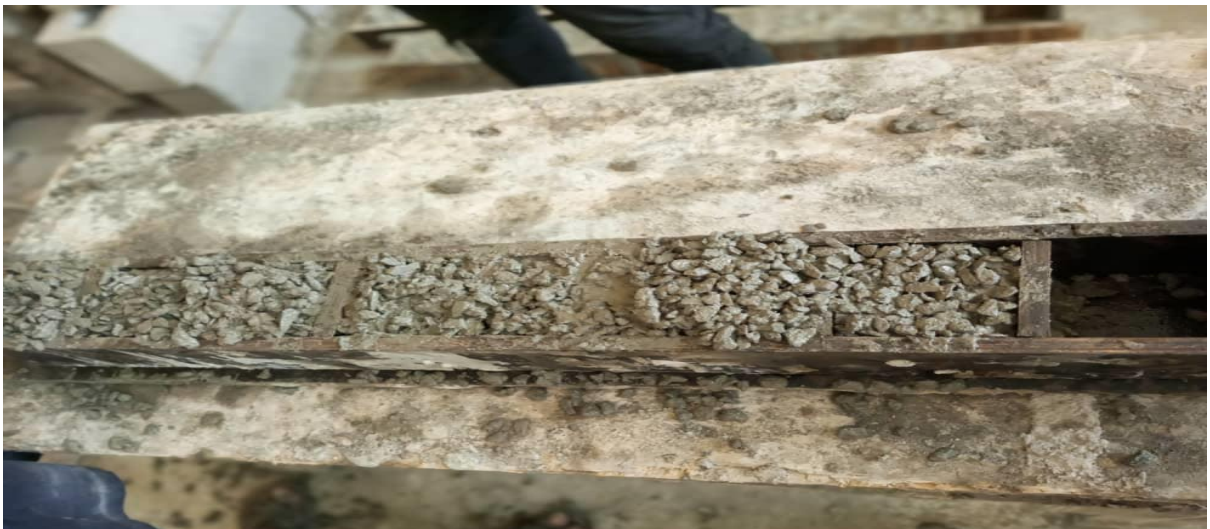
Figure 3.7: Casting and Vibration of concrete moulds.
