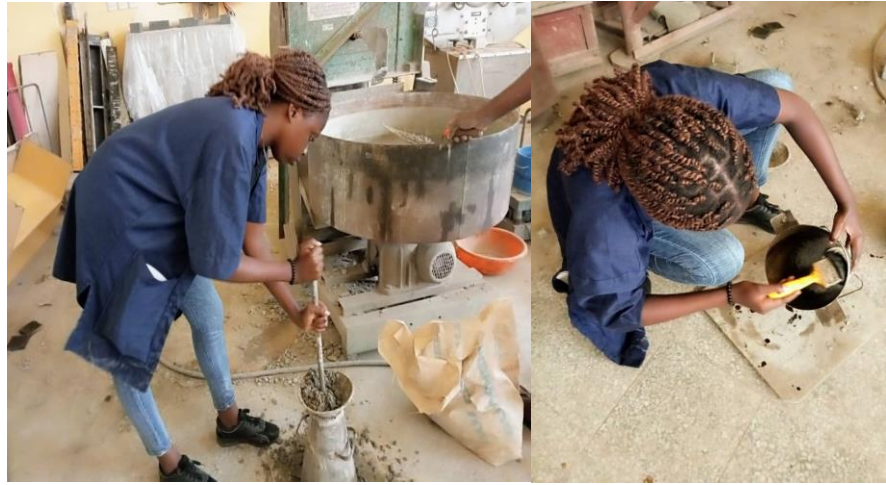
Figure 3.6: Slump Test carried out at the Structural Laboratory, Uniben.
