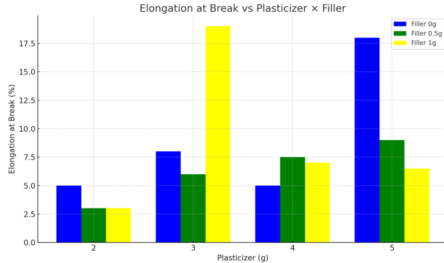
Fig 5: Elongation at break of CMS bioplastic film, using EG plasticizer and Kaolinite filler
