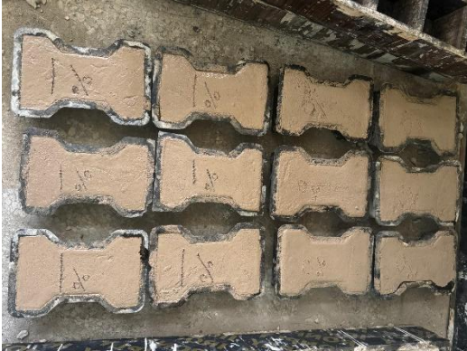
Sandcretes during casting
