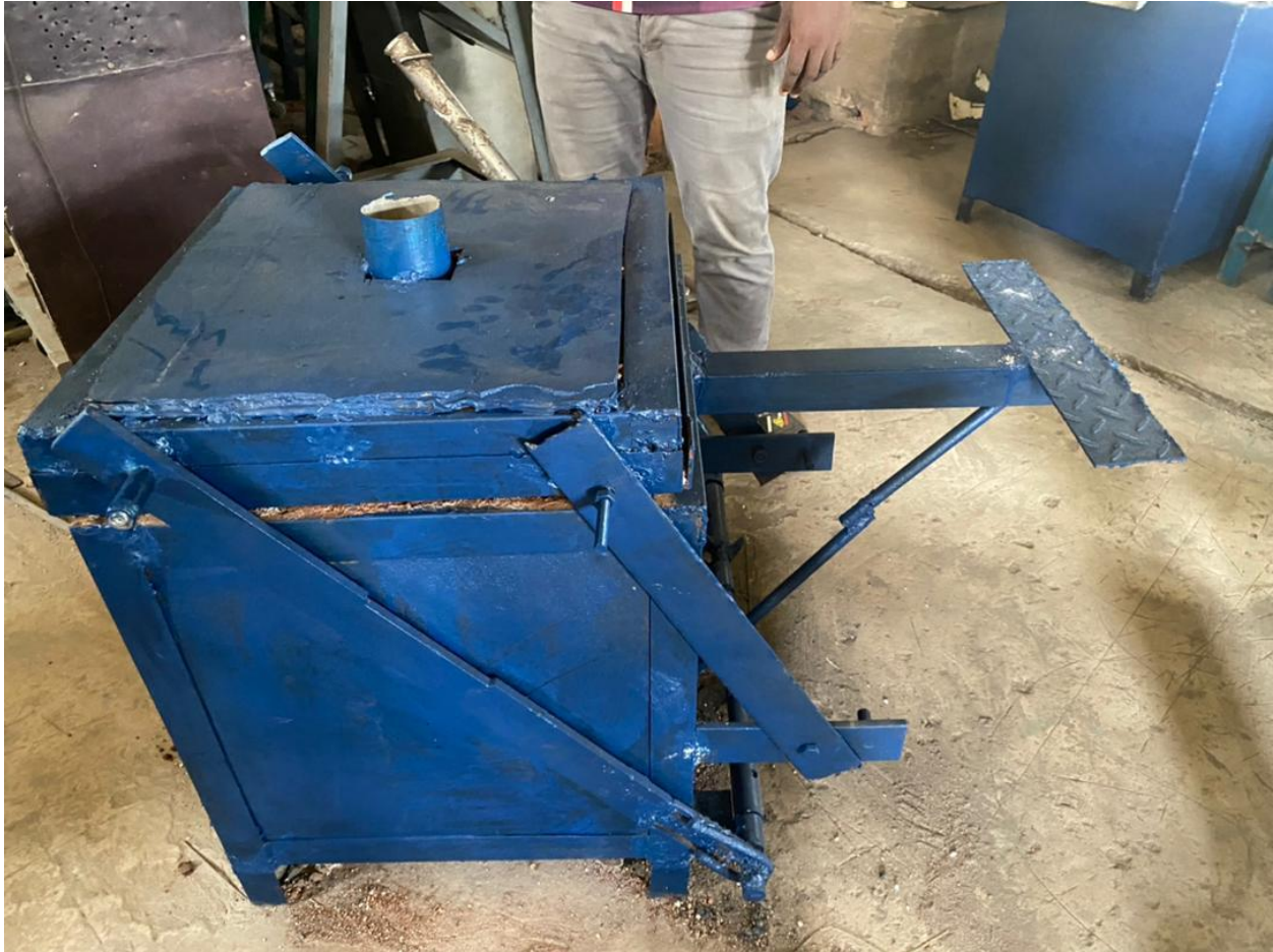
Fig. 3.5 Furnace cover and opening mechanism
