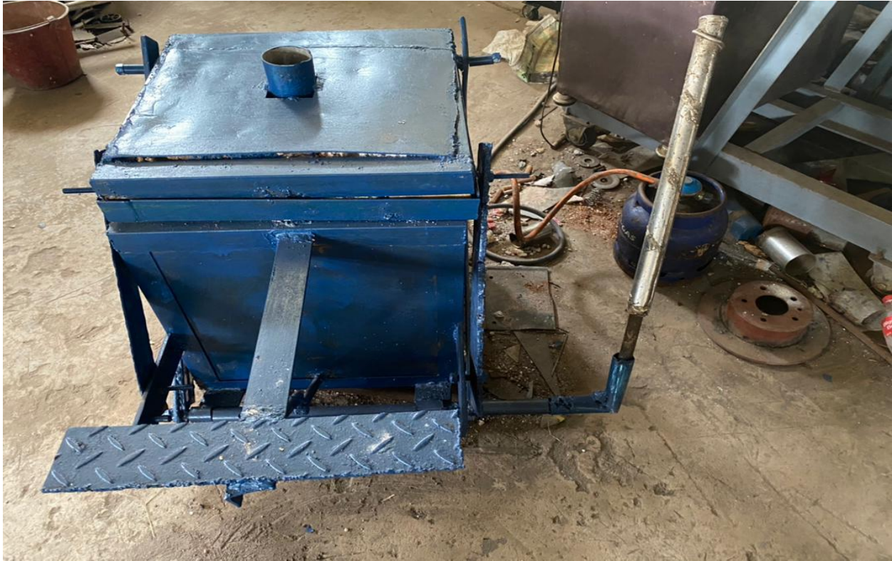
Fig 3.6 Assembled design of the crucible furnace
