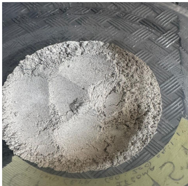
Plate 3.3: Catalyst Blend of Banana Peel Ash, Calcined periwinkle shell and Zeolite.
