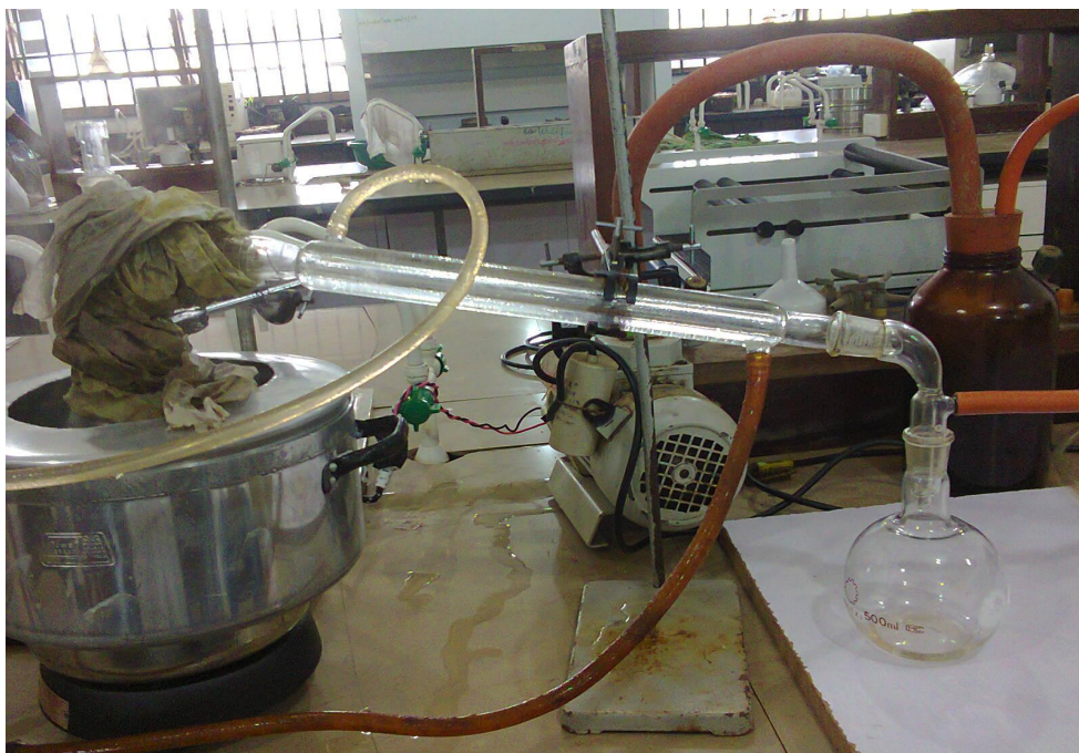
Plate 3: Vacuum Distillation Setup
