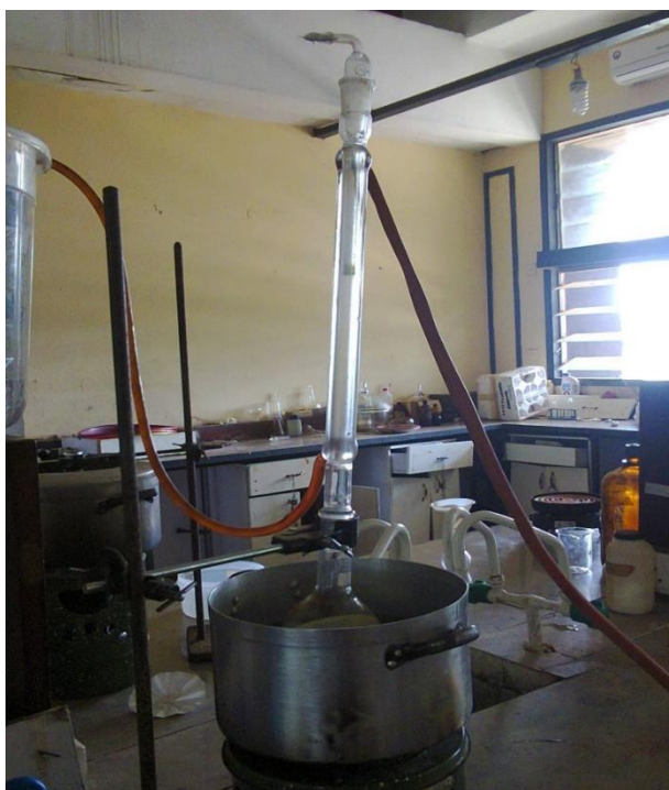
Plate 4: Setup for Refluxing
