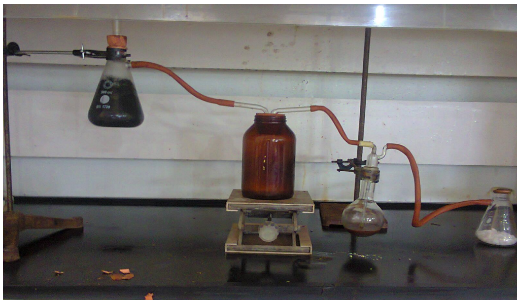
Plate 2: Passing \text{H}_2\text{S} through a Reaction Mixture of Compound 3 and Sodium ethoxide ( \text{C}_2\text{H}_5\text{ONa} )
