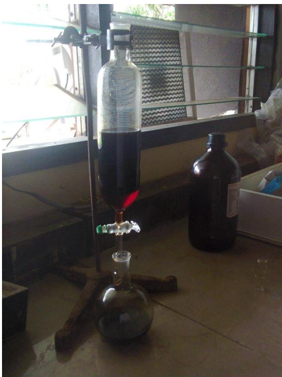
Plate 1: Extraction of Compound 2 using Chloroform
