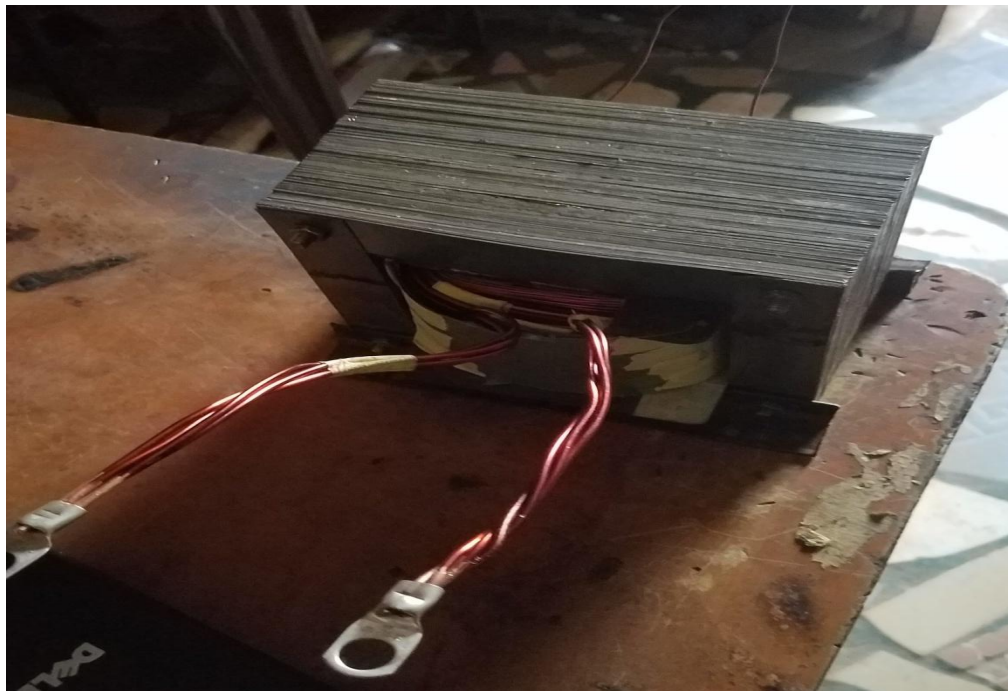
Fig. 4.4: the transformer after full assembly
