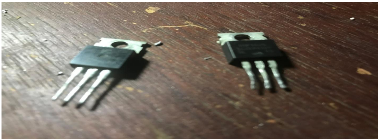
Fig. 4.3: the MOSFET IRF3205 used in the construction of the MOSFETs bank
