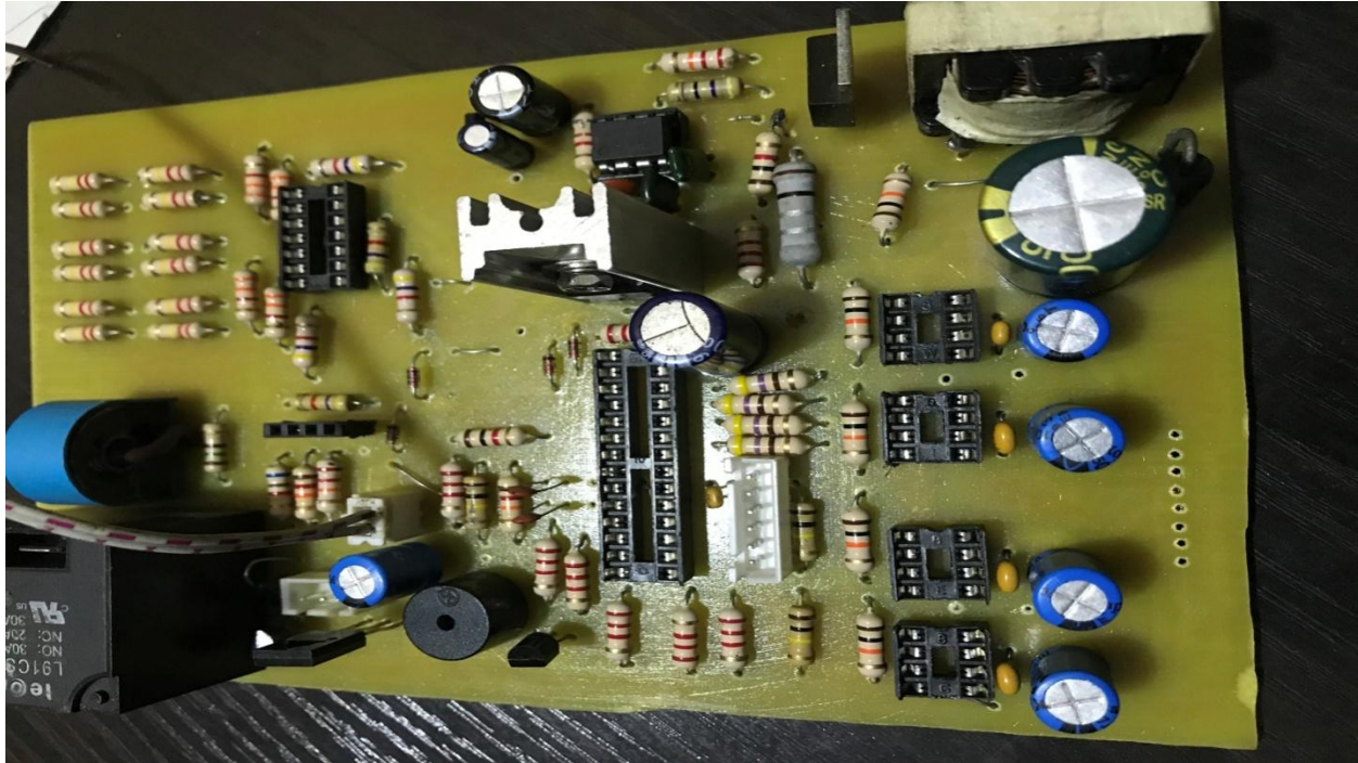
Fig. 4.1 (b) the control stage pcb after construction with components layout
