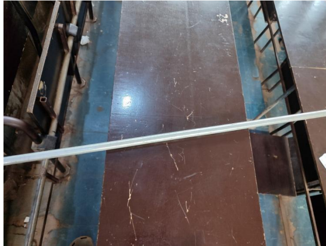
Figure 3.5 Rigid 0.5-inch PVC pipe for wand
