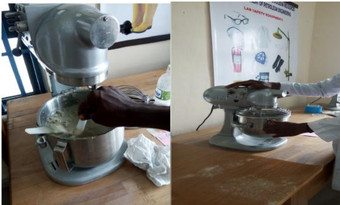
Fig. 1: Agitation Process of Water Base mud using Mud Mixer
