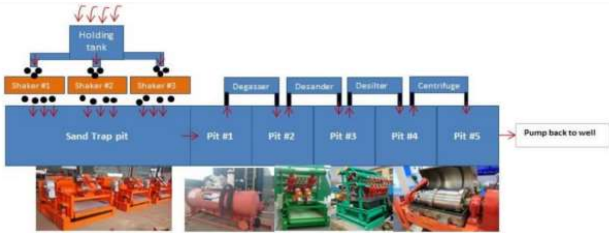
Figure 2.5 Solid Control System Process
