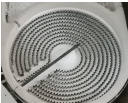
Figure 23 The Heat Generating Compartment
