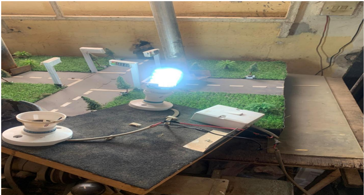
Fig 5.10: AC load in its ON state connected to the solar system
