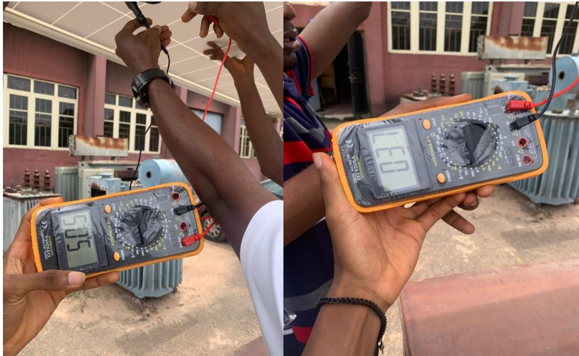
Fig 5.2: Short circuit current and open circuit voltage test using a multimeter
