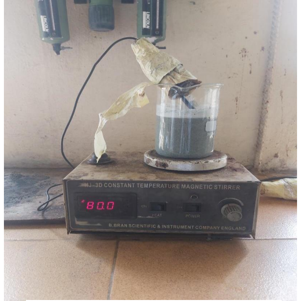
Wet Impregnation of catalyst and nickel nitrate precursor
