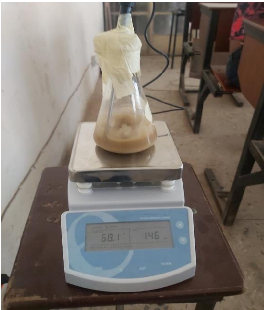
Simultaneous Esterification and Transesterification reaction using a Bi-functional catalyst
