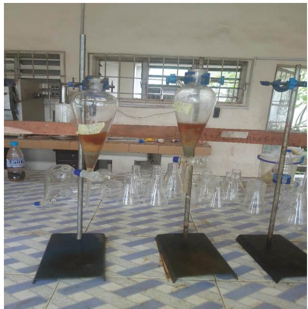
Wet Impregnation of catalyst and nickel nitrate precursor
