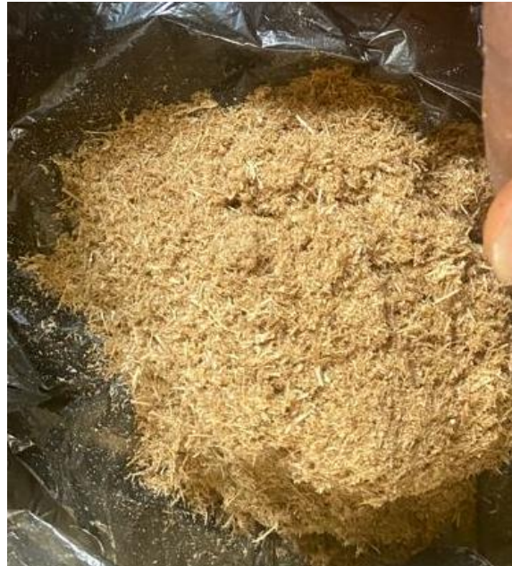
Plate 3.8: A sample of the grounded bamboo fibre
