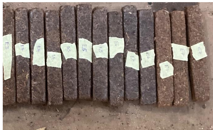
Plate 3.9: Samples of the full length of extracted composite specimens
