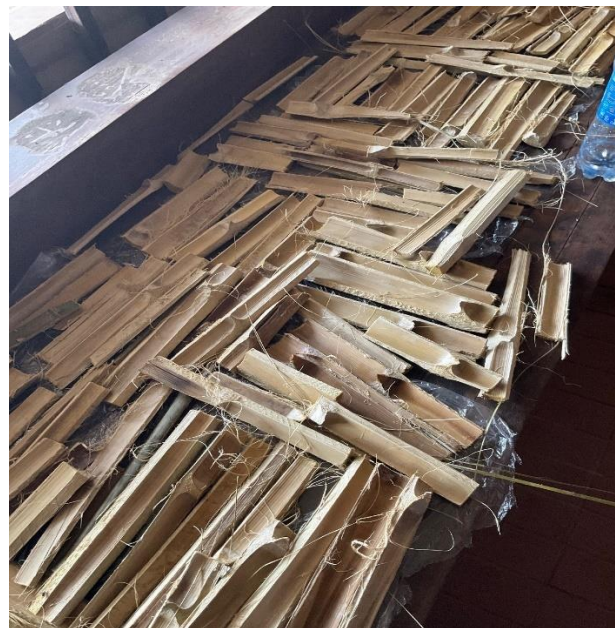
Plate 3.7: Air drying of the bamboo
