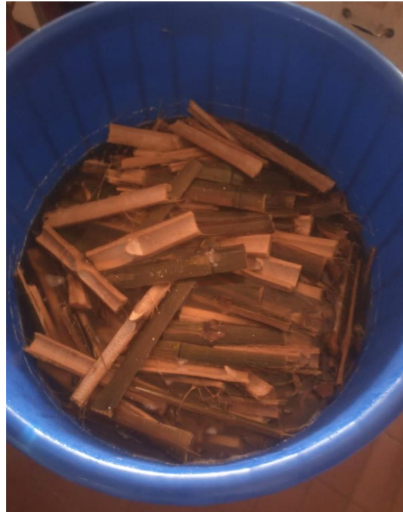
Plate 3.6: Delignification of bamboo
