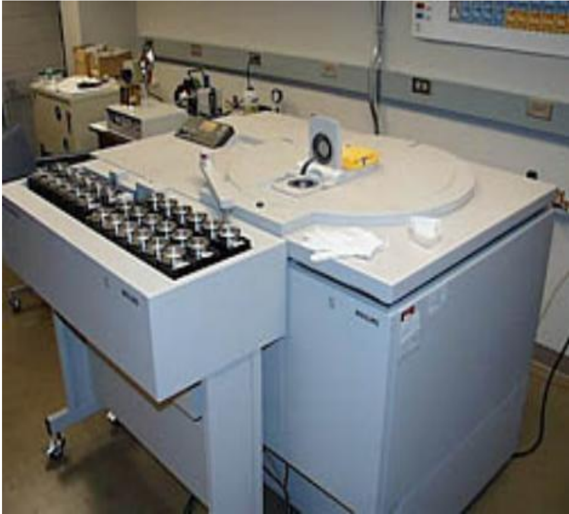
Plate 3.1: MODEL: TEFA ORTEC automatic X-ray Fluorescence Machine
