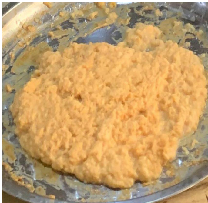
Fig 2.4. Showing the precipitated gum extract from ( Chrysophyllum albidum ) juice
