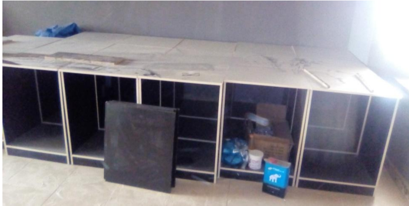
PLATE 12 TITLE: BOARDS FOR LIGHT BOX AND LOCKERS COUPLED TOGETHER SOURCE: TEXTILE STUDIO PHOTOGRAPH: AZIH EMMANUEL
