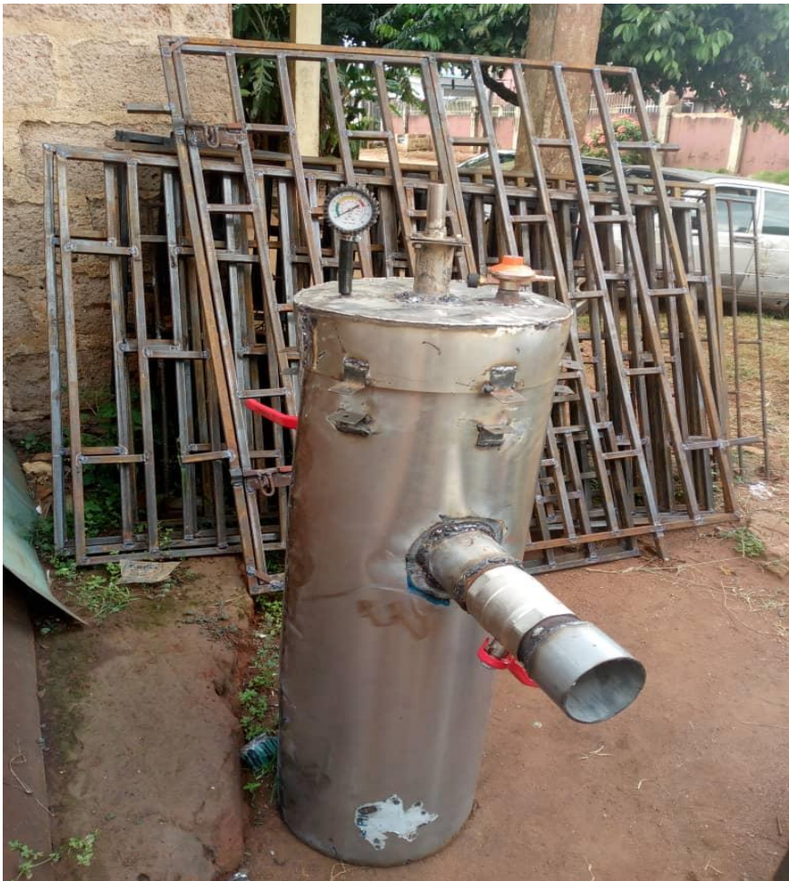
Figure 4.6 - fully assembled biogas digester
