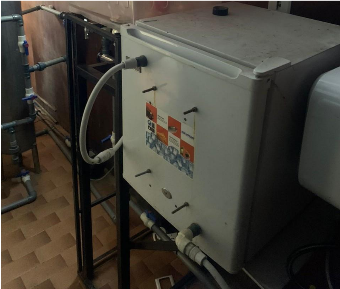
Figure 3.5: Refrigerator and Heater Stations
