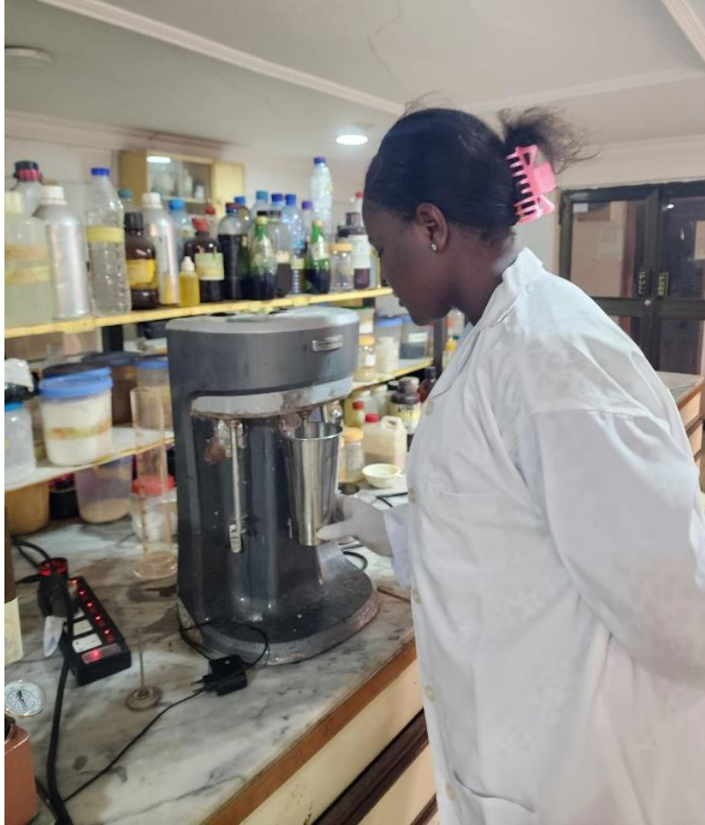
PLATE 3.1: Mud Preparation and Mixing
