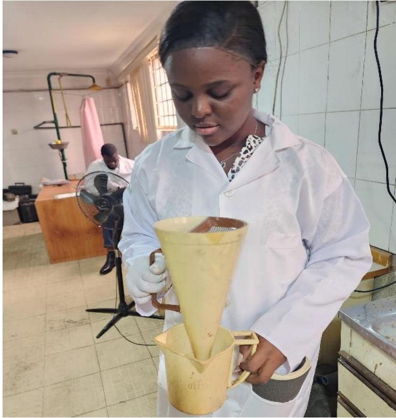
PLATE 3.3: Rheological Property Measurements (Viscosity)
