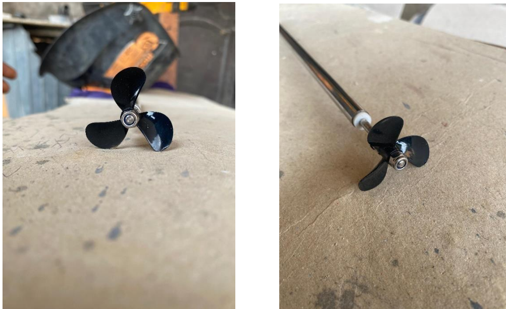
Fig 3.2 Plastic propeller with 30cm shaft.
