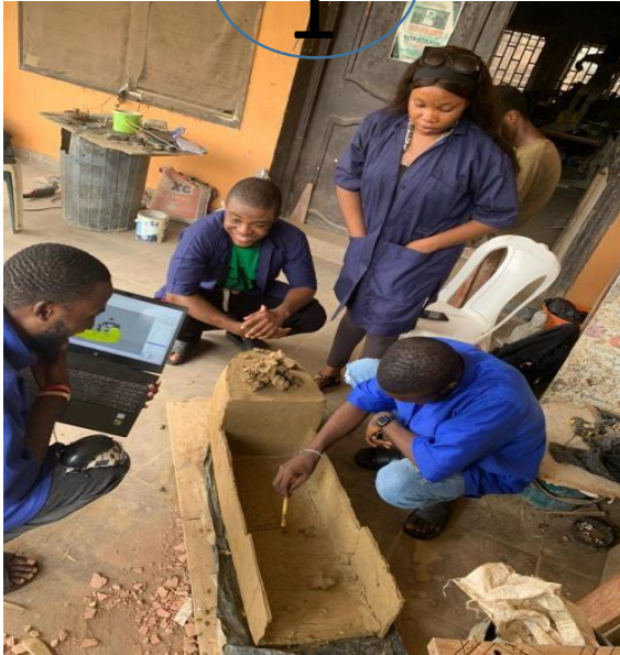
Getting Mold of Ship Hull using Clay
