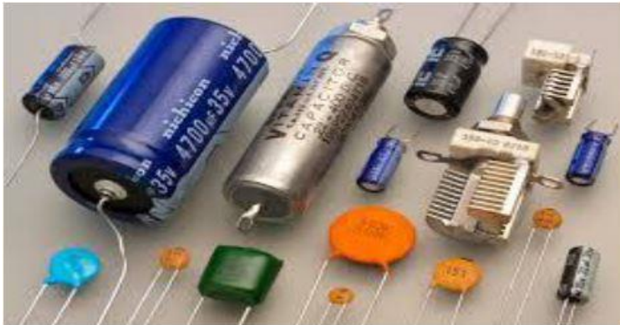
Figure 3.4: Different types of capacitors (Wikipedia, 2023)
