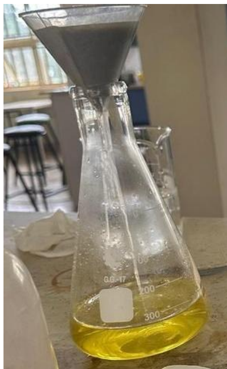
Plate 3.5 Washing the acid-activated clay with distilled water to achieve neutral pH.
