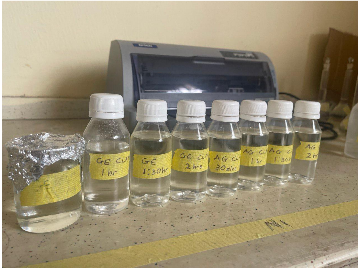
Plate 3.9 Digested produced water samples prepared for analysis via Atomic Absorption Spectrophotometry (AAS).
