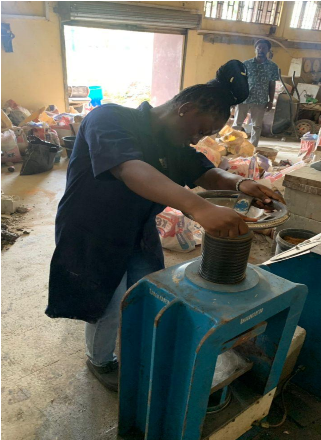
Fig 1; Preparing the crushing machine to crush cubes that have been cured.
