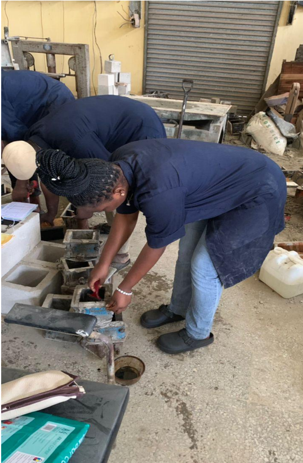
Fig 2; Lubricating of moulds before filling with concrete mix.
