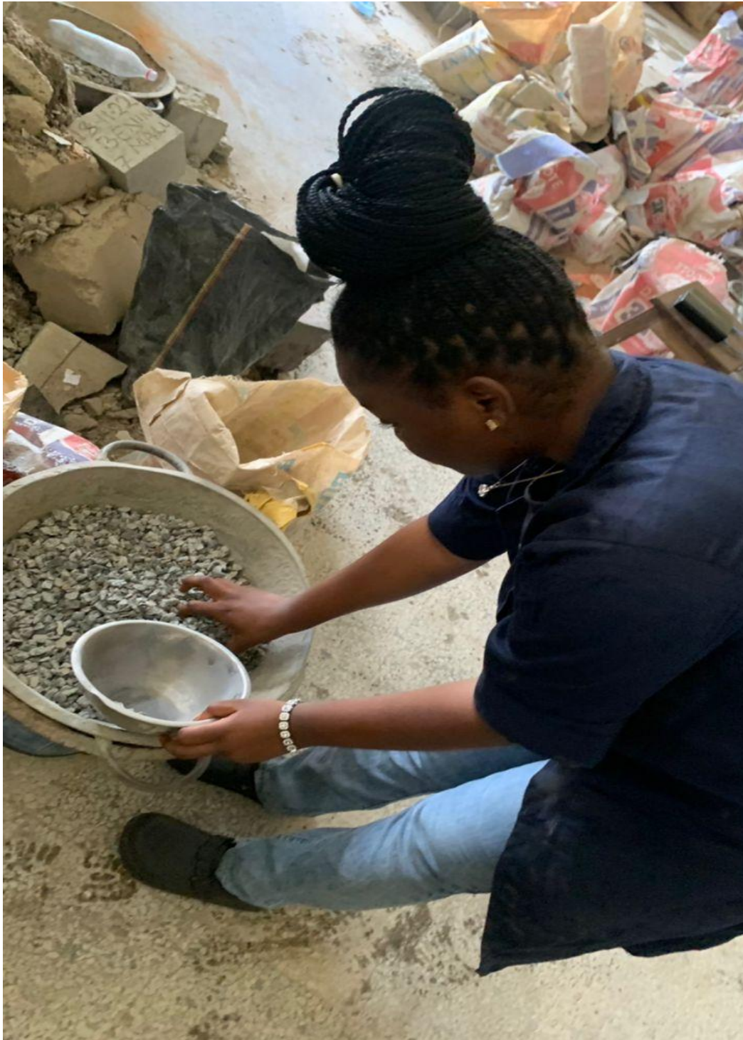
Fig 3; Packing coarse aggregates to measure them for concrete mix.
