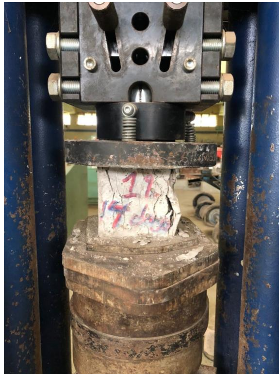
Plate B 3 Specimen inside compressive strength machine
