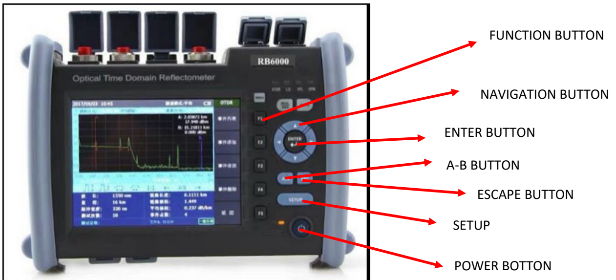
Figure 3.3: Front view of the OTDR
